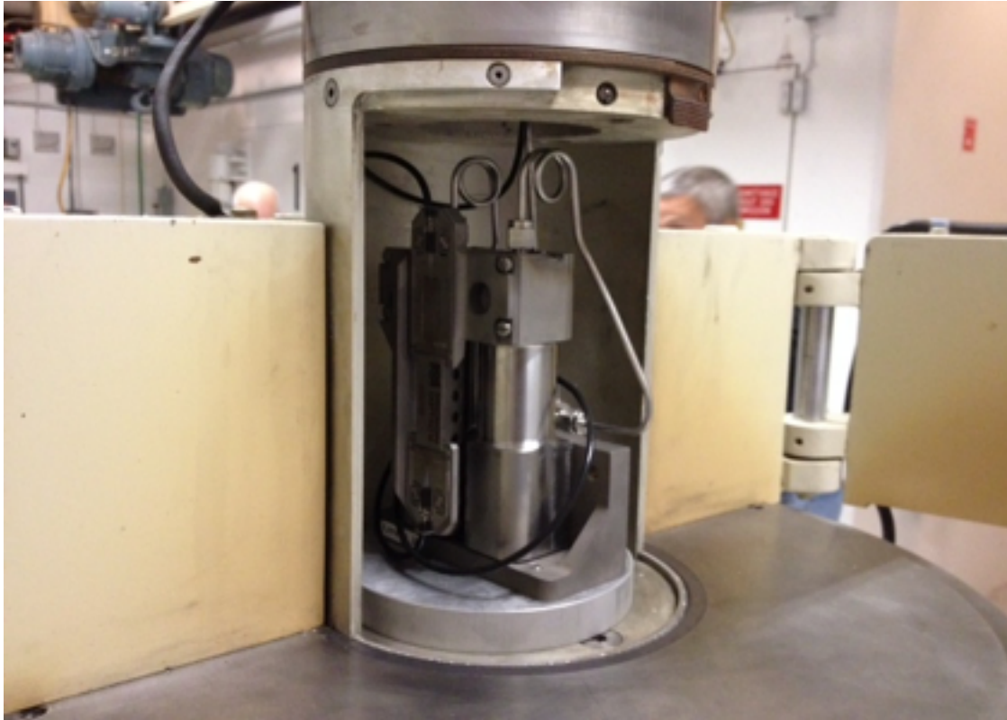
FIGURE 2: The core components of the optical fiber pressure sensor were mounted in the Gammacell 200 for irradiation testing.
