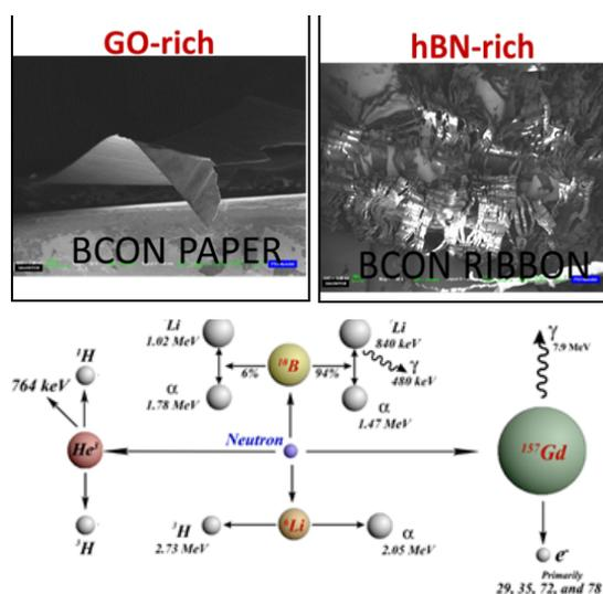
FIGURE 2: BCON paper, BCON ribbon, and boron interactions with neutrons, producing gamma-rays and alpha particles [3].
