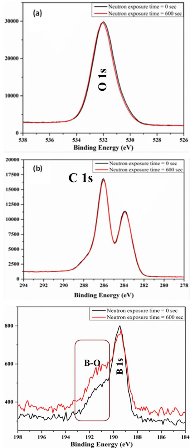
**FIGURE 4: Changes in the high resolution spectra for (a) O 1s and (b) C 1s showing a minimum change in the peak structure indicating that there was no change before and after the neutron exposure. (c) A slight change in B 1s indicating that the concentration of boron atoms should be higher in order to see any statistically significant change.**
