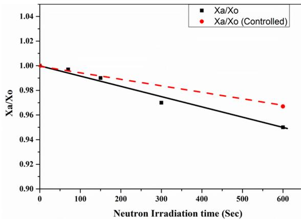
**FIGURE 3: XPS measurement of the O/C ratio for GO after thermal neutron irradiation and a control sample.**
