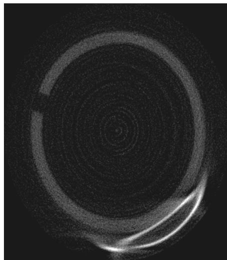
**FIGURE 3: Sample aluminum cylinder with copper tubing wrapped around cross section information (361 projections in 180° at 0.2 s/frame)**
