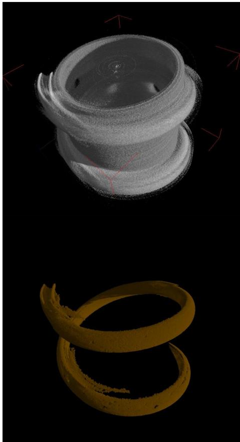
**FIGURE 4:** Volume reconstruction results of the aluminum cylinder with copper tubing wrapped around detailed internal information using VG-Studio Max.1.2
