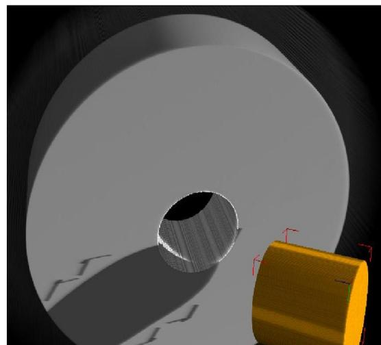
**FIGURE 6:** Visualization of the aluminum cylinder with copper core 3-D information using VG-Studio Max
